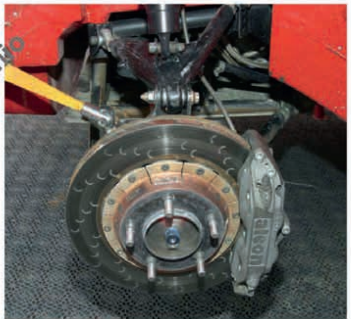
Double wishbone suspension design is by Epsilon, using Sachs coilovers. Alcon discs are limited to 310mm to allow the use of 15in wheels in the wet
