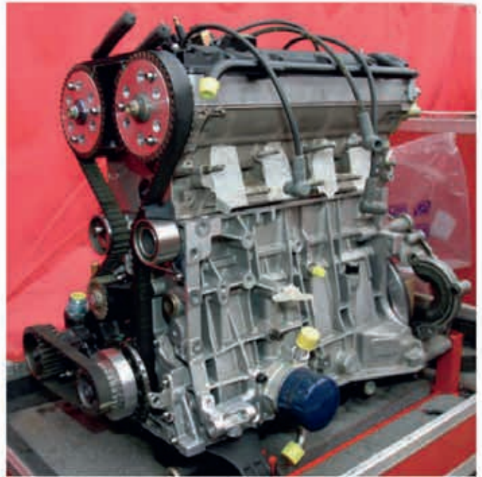
Oreca-prepared engine uses alloy XU7 block and 16v head from 1.8-litre Xsara
