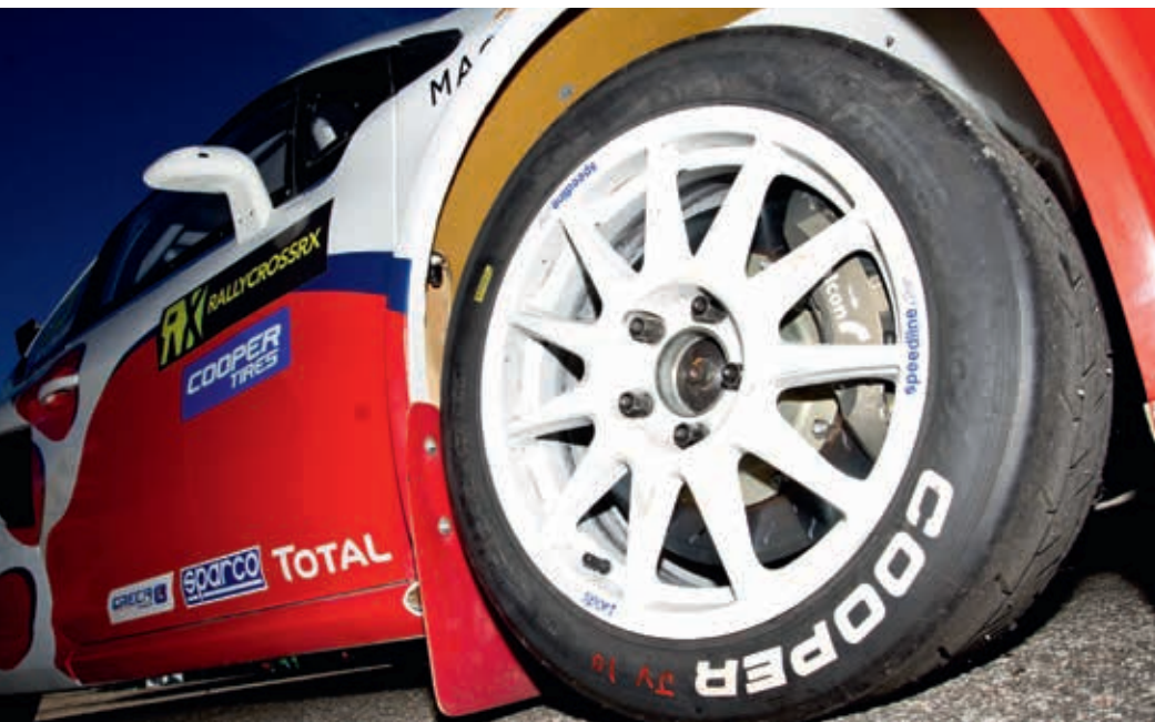
RX tyres don't use kerbing ribs in a bid to save weight, but they do feature layers of Kevlar and nylon for strength
