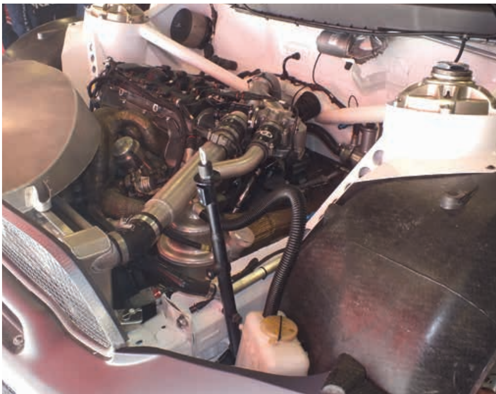
Top: The RX MINI uses an S2000 asphalt brake setup with gravel spec discs and calipers on the rear Above: Engine bay is already extremely cramped and would struggle to accommodate a 2.0-litre powerplant
