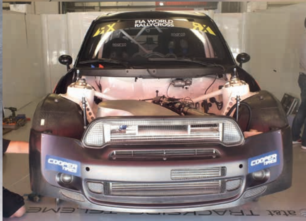
Top: The cooling fans can clearly be seen – these play a huge role in keeping performance consistent
