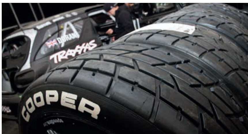
The tyres must be constructed so that they can be hand cut from slicks to intermediates to wets
